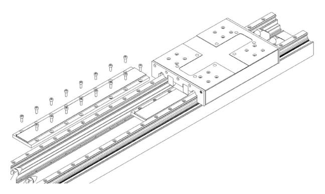
8. Test whether the motor moves without contact with the magnetic ways over the whole magnetic way. It is normal to observe variations in the forces depending on the position (detent force).
