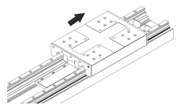
7. Mount and fix the remaining magnetic plate segments with the fixing screws.
