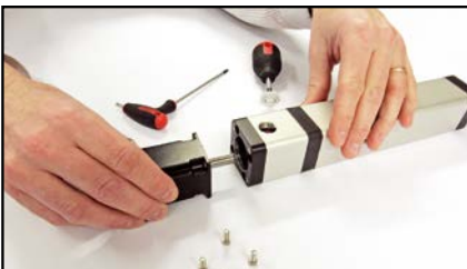
Insert motor shaft into coupling
